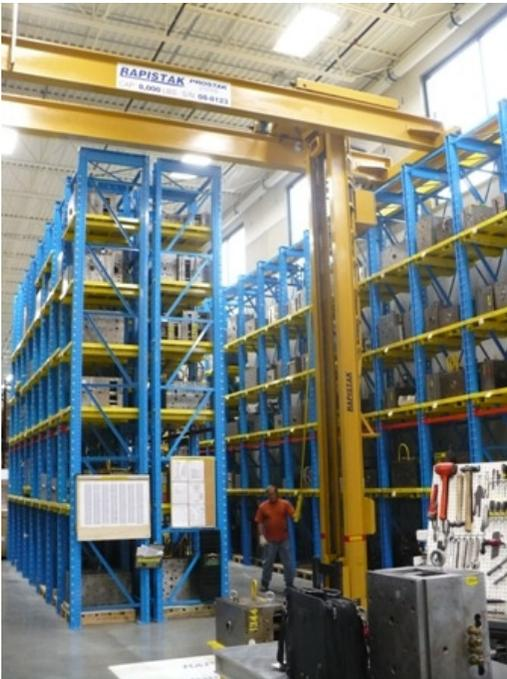
Stacker storage systems can be as short as 10 feet and as tall as 25 feet. These systems can be configured as single aisle, double aisle and even triple aisle systems. For rack mounted stacker storage systems mold or die capacity can go up to 8,000 pounds. When higher capacities up to 25,000 pounds are required free standing support systems or existing runway systems are used in conjunction with the rack systems to provide a complete storage system.
